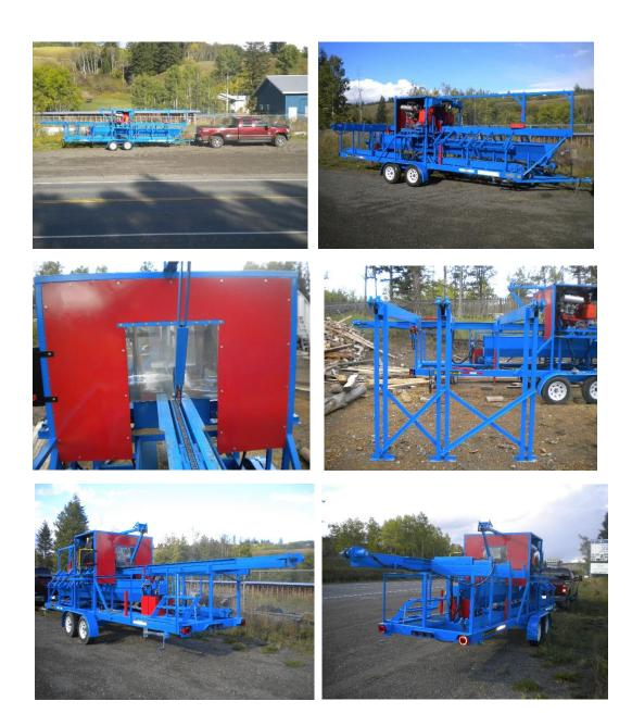
Thank you for your interest in our products. The D&L Small Log Scragg was design to be portable to take the mill to the wood. It is easy to set up and is manufactured with off the shelf parts. Our mill runs with 3 people and a small loader skid steer will work with this mill lower the initial capital costs.
